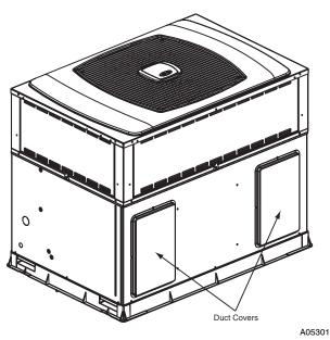
Fig. 11 - 50CR with Duct Covers On
